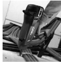
Conduits & pipes with metal or textile band
