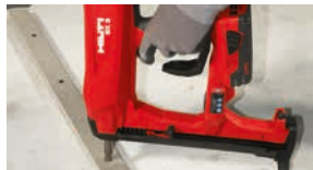
Fastening wood, e.g. Placopan®, to concrete
