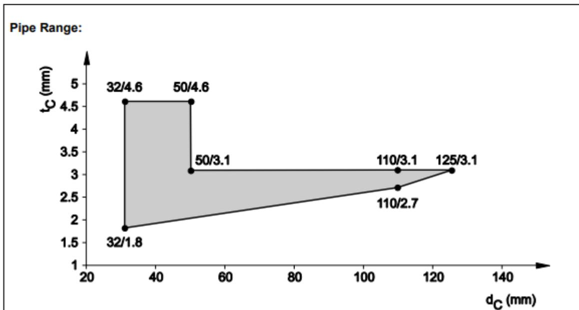
8.3.2.6 PE pipes acc. EN 15494, EN 12201-2 and DIN 8074/75 in flexible wall ( $t_E \geq 100$  mm), pipe group 1, EI 120 - U/C
