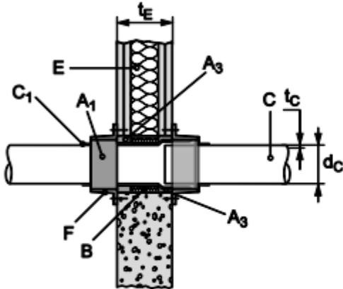
Requested number of hooks on CFS-C EL to seal pipes, penetrating a flexible wall/ rigid wall ( $t_E \geq 100$ mm) and using a linear pipe coupling. (no elbow). If pipe insulation thickness is between 0 and 4 mm use the number of hooks indicated for 4 mm. If pipe insulation thickness is between 4 and 9 mm use the number of hooks indicated for 9 mm.
