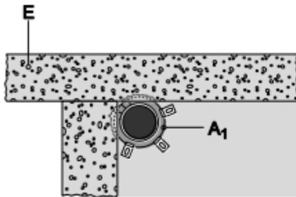
8.4.2.20 PE pipes acc. EN 1519-1, EN 12201-2 and EN 12666-1, in rigid wall ( $t_E \geq 150$  mm), pipe group 2, EI 120 - U/U
