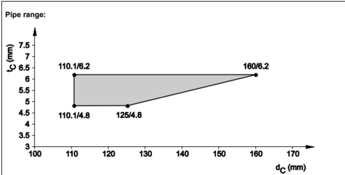
8.5.2.16 ABS pipes acc. EN 1455-1, EN 15493 and SAN+PVC-pipes acc. EN 1565-1, in rigid floor ( $t_E \geq 150$  mm), pipe group 2, EI 120 - U/U
