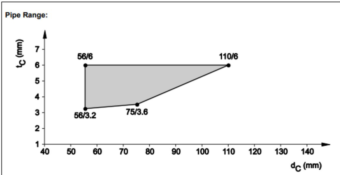
8.3.2.13 PVC-pipes, non-regulated (Friatec Friaphon), in flexible wall ( $t_E \geq 100$  mm), pipe group 1, EI 90 - U/U
