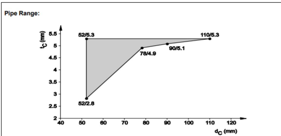
8.3.2.14 Pneumatic dispatch system, PVC pipe acc. DIN 6660, in flexible wall ( $t_E \geq 100$  mm), pipe group 1, EI 90 - U/U
