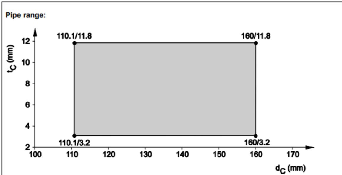
8.5.2.22 PP pipes, non-regulated, in rigid floor ( $t_e \geq 150$  mm), pipe group 2, EI 120 - U/U
