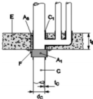
8.5.2.46 PP pipes acc. EN 1451-1 and DIN 8077/78 in rigid floor ( $t_E \geq 150$  mm), pipe group 1, EI 120 - U/U, Pipe coupling
