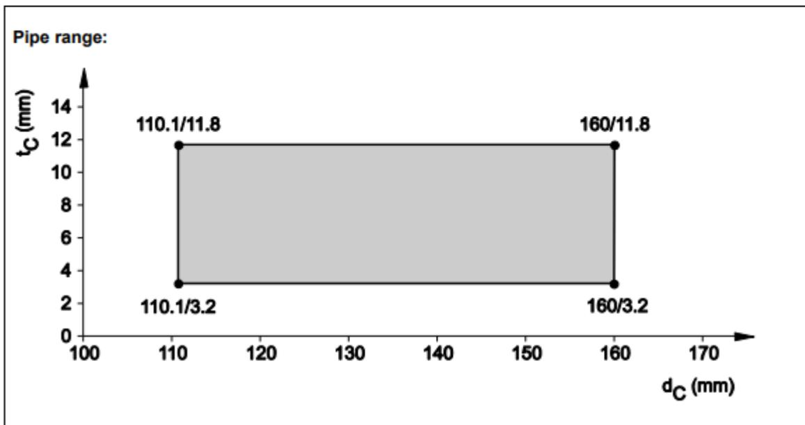
8.5.2.27 PVC pipes, non-regulated (Friatec Friaphon), in rigid floor ( $t_E \geq 150$  mm), pipe group 2, EI 180 - U/U
