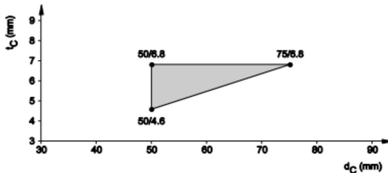
8.4.2.17 PP pipes, non-regulated, gap sealed with CFS-FIL, in rigid wall ( $t_e \geq 100$  mm), pipe group 1, EI 90 - U/U, elbow pipe 87°
