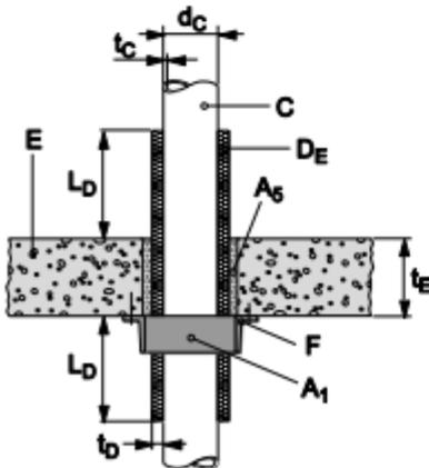
8.5.2.29 **PP-R - pipes acc. EN 15874 (Aquatherm fusiolen = aquatherm green pipe S), insulated, in rigid floor ( $t_E \geq 150$  mm), pipe group 1, EI 120 - U/C**
