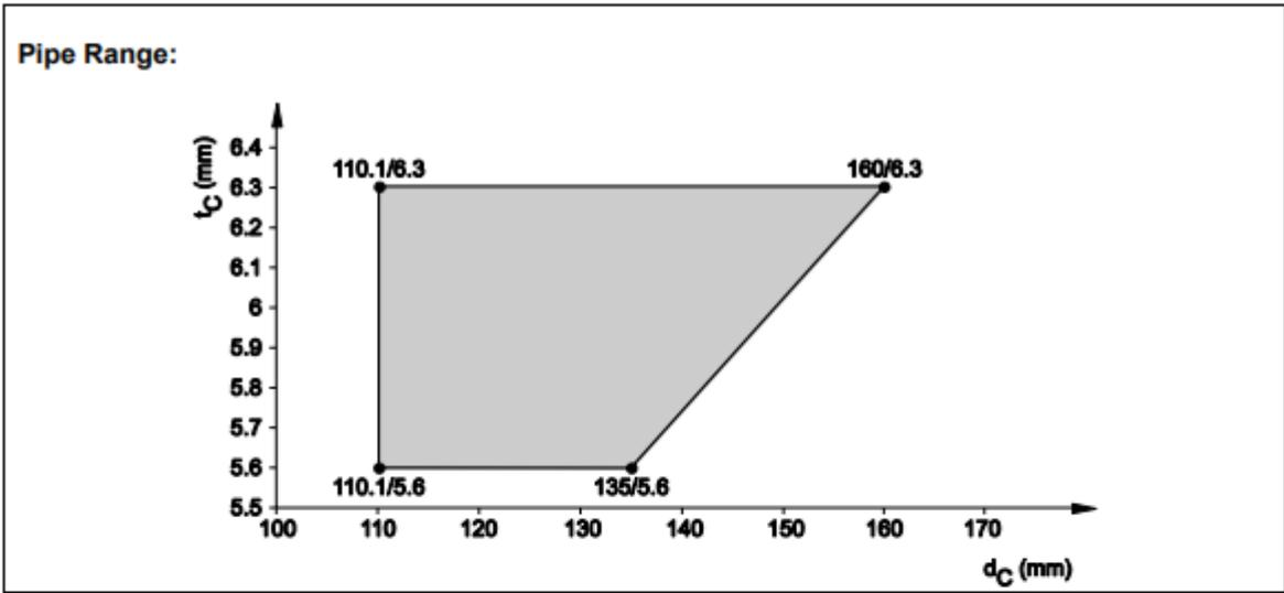
8.5.2.28 PE-X - pipes acc. EN 15875 (Rehau Rautitan flex), insulated, in rigid floor ( $t_E \geq 150$  mm), pipe group 1, EI 120 - U/C
