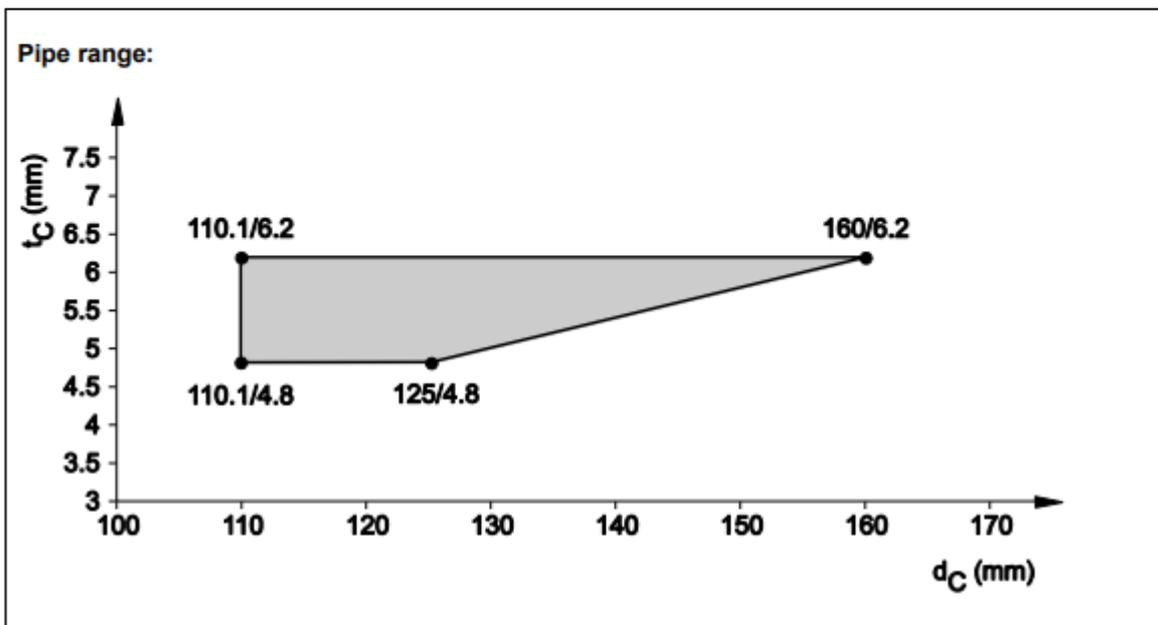
8.5.2.17 ABS pipes acc. EN 1455-1, EN 15493 and SAN+PVC-pipes acc. EN 1565-1, in rigid floor ( $t_E \geq 150$  mm), pipe group 2, EI 60 - U/U
