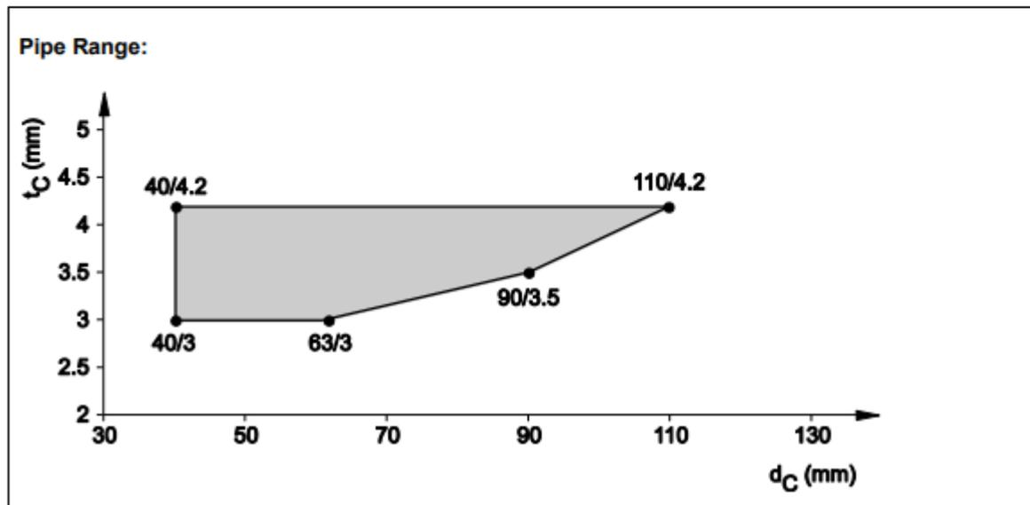
8.4.2.2 PE pipes acc. EN15494, EN 12201-2 and DIN 8074/75, in rigid wall ( $t_E \geq 100$  mm), pipe group 1, EI 120, U/U
