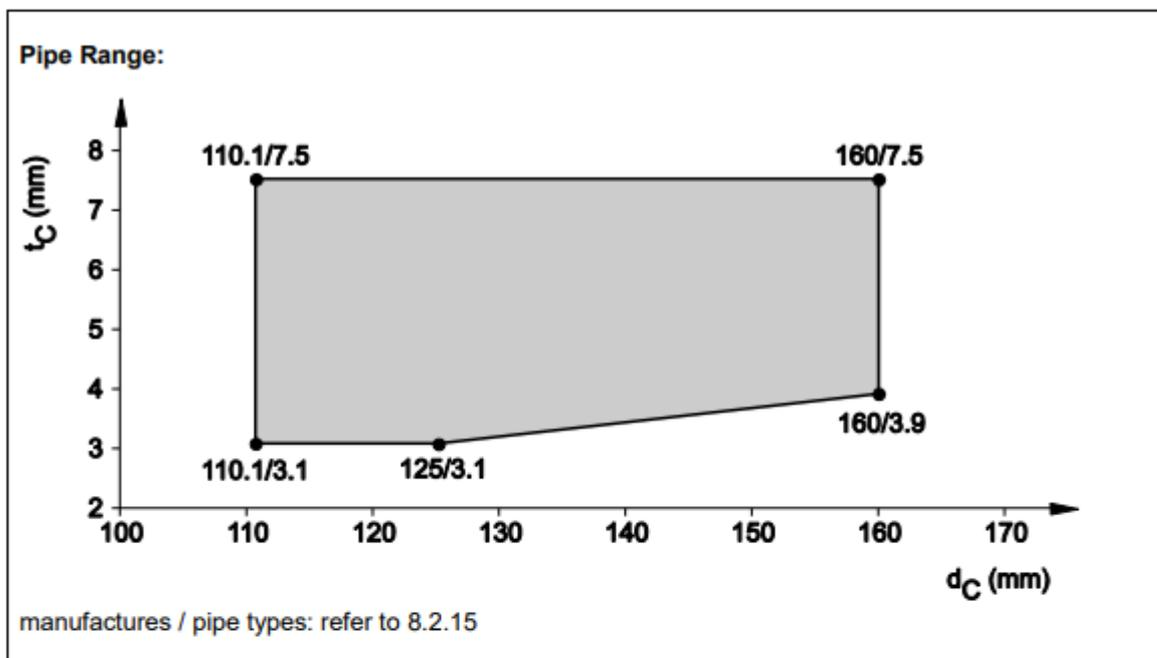
8.4.2.26 PP pipes acc. EN 1451-1 and DIN 8077/78, in rigid wall ( $t_E \geq 150$  mm), pipe group 2, EI 120 - U/U
