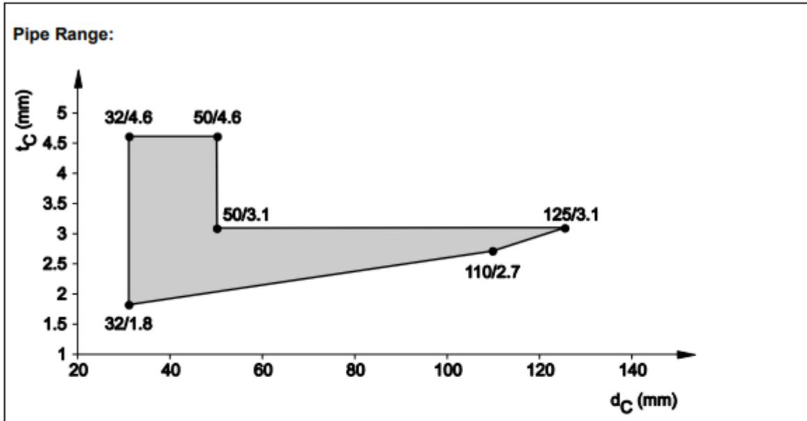
8.4.2.3 PE pipes acc. EN15494, EN 12201-2 and and DIN 8074/75, in rigid wall ( $t_E \geq 100$  mm), pipe group 1, EI 120 - U/C
