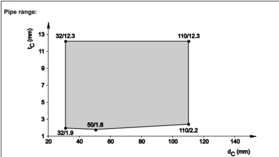
8.5.2.5 PVC pipes acc. EN 1452-1, EN 1329-1, EN 1453-1, EN 1566-1, EN ISO 15493 and DIN 8061/62, in rigid floor ( $t_e \geq 150$  mm), pipe group 1, EI 90 - U/U
