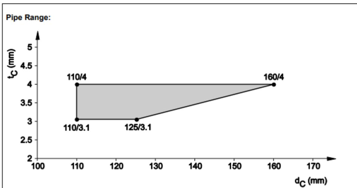
8.4.2.27 PP pipes acc. EN 1451-1 and DIN 8077/78, in rigid wall ( $t_E \geq 150$  mm), pipe group 2, EI 30 - U/U
