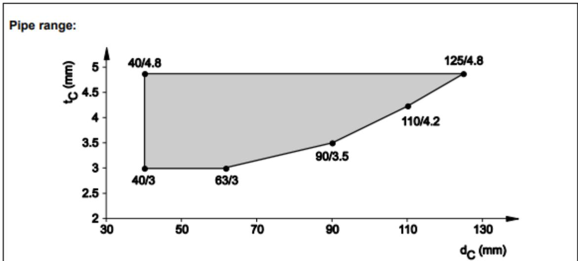
8.5.2.2 ABS pipes acc. EN 1455-1, EN 15493 and SAN+PVC-pipes acc. EN 1565-1, in rigid floor ( $t_E \geq 150$  mm), pipe group 1, EI 120 - U/U
