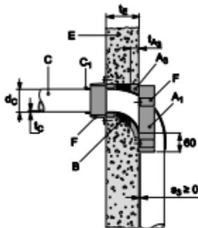
**8.4.2.18 PP pipes, non-regulated, gap sealed with CFS-FIL, in rigid wall ( $t_e \geq 100$  mm), pipe group 1, EI 120 - U/U, elbow pipe 2 x 45°**
