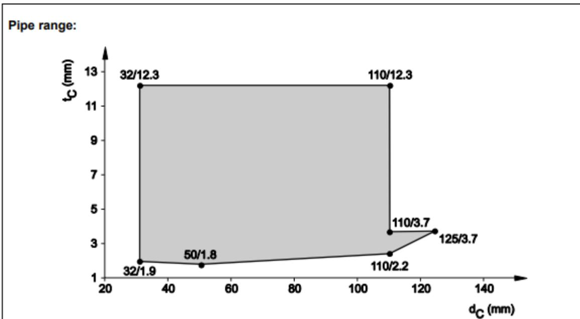
8.5.2.6 PP pipes, non-regulated, pipe types: refer to 8.2.15, in rigid floor ( $t_E \geq 150$  mm), pipe group 1, EI 120 - U/U
