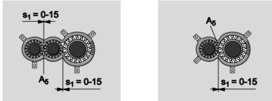
**8.5.2.31 Reuse of oddments of CFS-C EL, in rigid floor ( $t_E \geq 150 \text{ mm}$ ), pipe group 1 and 2, EI 120 - U/U****Situation:**
