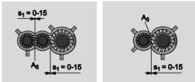
8.4.2.10 Multiple pipe penetration, covered with foamed elastomeric thermal insulation, in rigid wall ( $t_E \geq 100$  mm), pipe group 1, EI 120 - U/C, zero distance to floor basement
