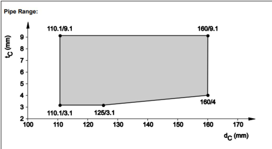
8.4.2.28 PP pipes acc. EN 1451-1 and DIN 8077/78, in rigid wall ( $t_E \geq 150$  mm), pipe group 2, EI 120 - U/C
