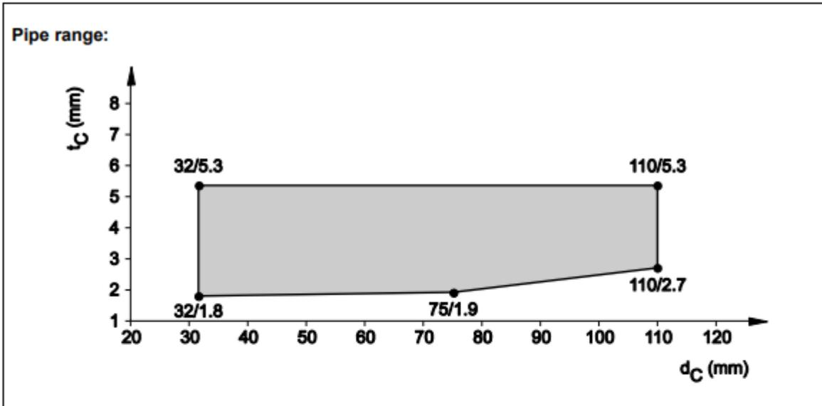
8.5.2.7 PP pipes acc. EN 1451-1 and DIN 8077/78, in rigid floor ( $t_E \geq 150$  mm), pipe group 1, EI 120 - U/U
