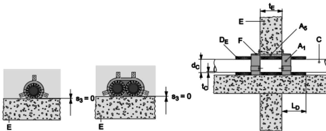
8.4.2.11 Roof drainage, covered with foamed elastomeric thermal insulation, in rigid wall ( $t_E \geq 100$  mm), pipe group 1, EI 90 or EI 120 - U/U
