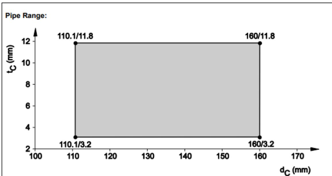
8.4.2.25 PP pipes, non-regulated, in rigid wall ( $t_E \geq 150$  mm), pipe group 2, EI 120 - U/U
