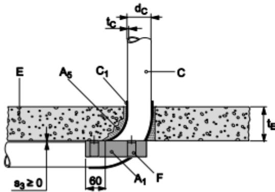
8.5.2.35 All PP pipes non-regulated, in rigid floor ( $t_E \geq 150$  mm), pipe group 1, EI 120 - U/U, elbow pipes 2 x 45°
