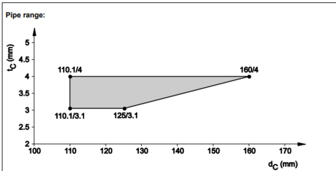
8.5.2.21 PVC pipes acc. EN 1452-1, EN 1453-1, EN 1566-1, EN 1329-1, EN ISO 15493 and DIN 8061/62, in rigid floor ( $t_e \geq 150$  mm), pipe group 2, EI 90 - U/U
