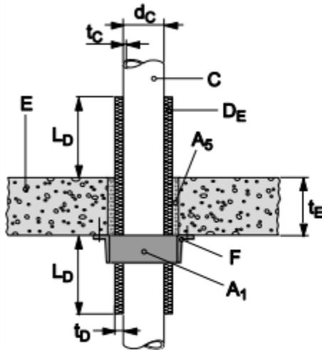
8.5.2.30 **Multiple penetration, thermal insulated, in rigid floor ( $t_E \geq 150$  mm), pipe group 1, EI 120 - U/U and U/C**
