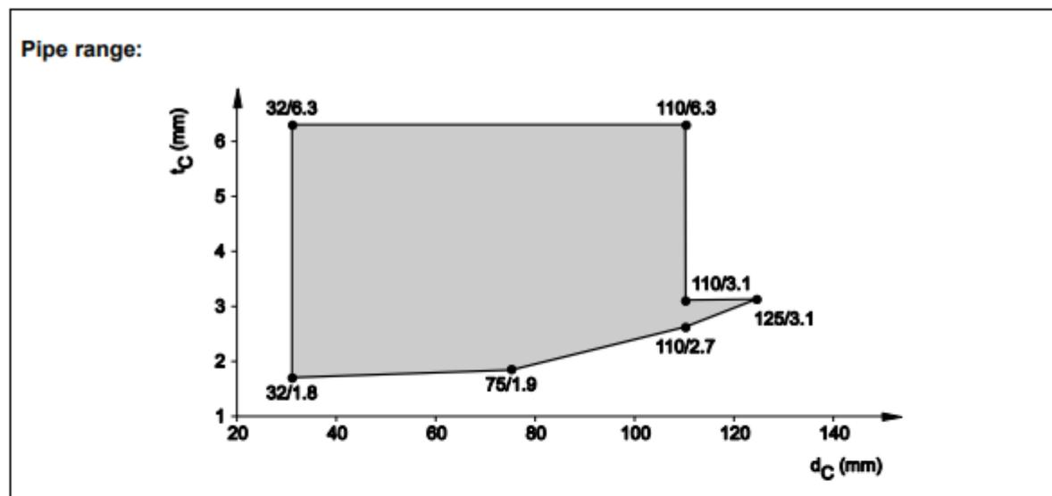
8.5.2.9 PP pipes acc. EN 1451-1 and DIN 8077/78, in rigid floor ( $t_E \geq 150$  mm), pipe group 1, EI 120 - U/C
