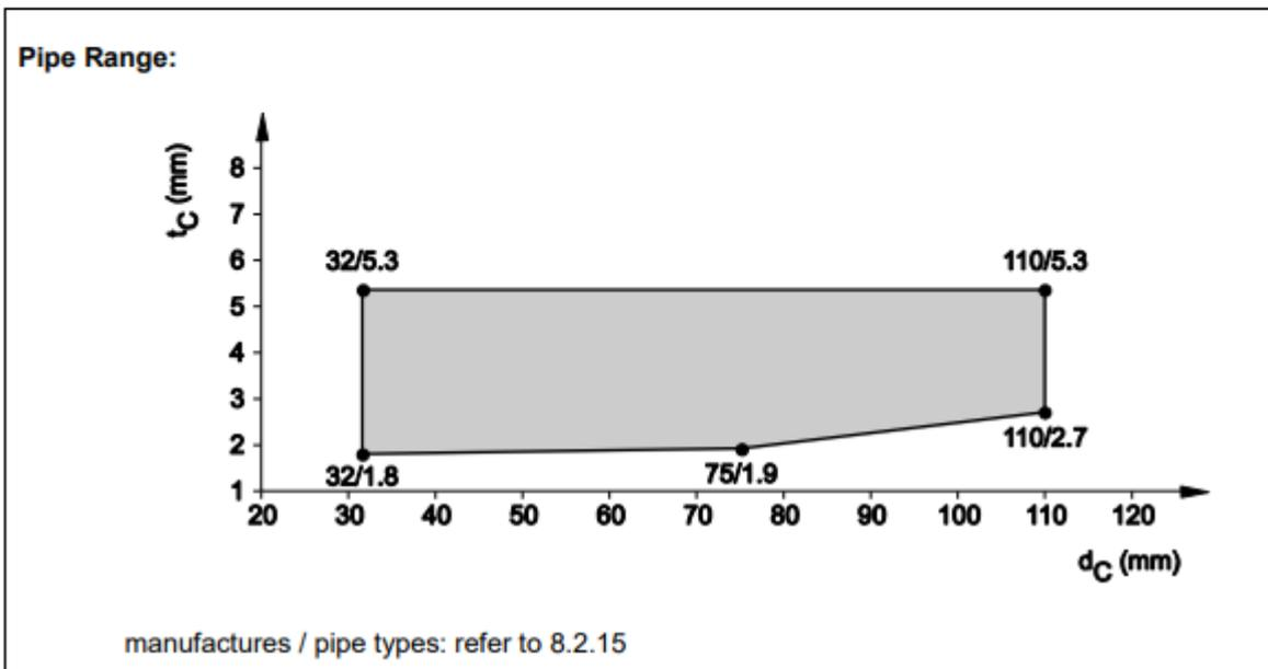
8.3.2.10 PP pipes acc. EN 1451-1 and DIN 8077/78, in flexible wall ( $t_E \geq 100$  mm), pipe group 1, EI 120 - U/U
