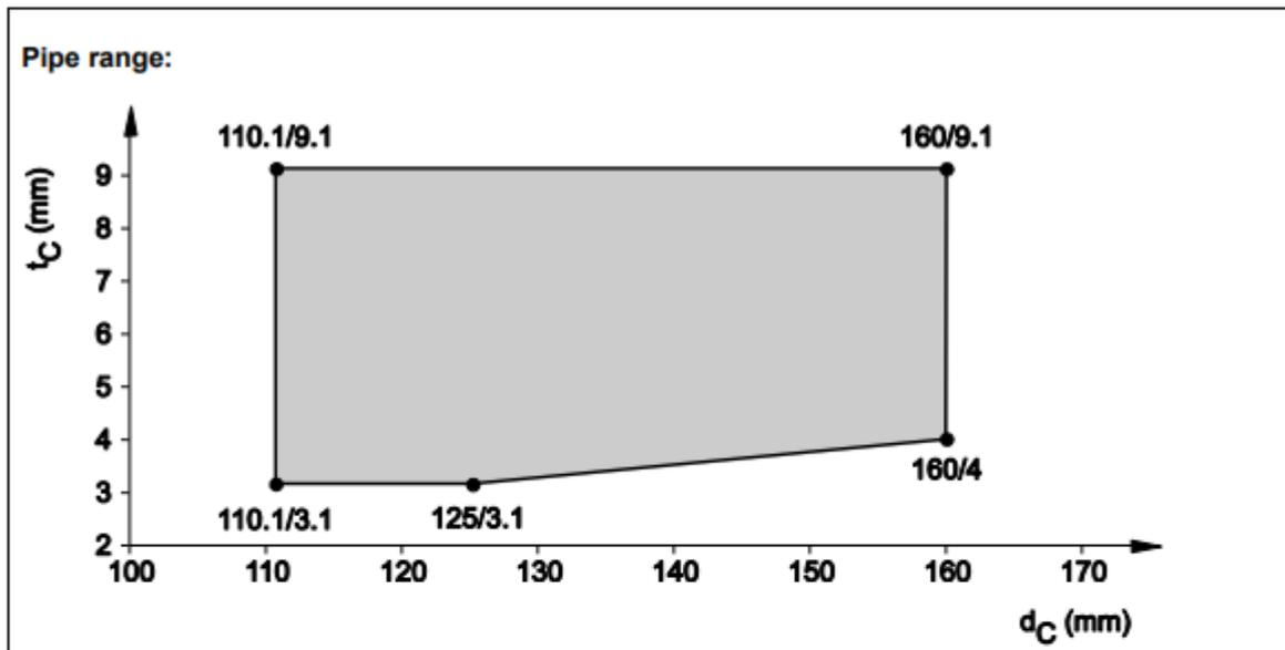
8.5.2.20 PE pipes acc. EN 15494, EN 12201-2 and DIN 8074/75, in rigid floor ( $t_E \geq 150$  mm),
