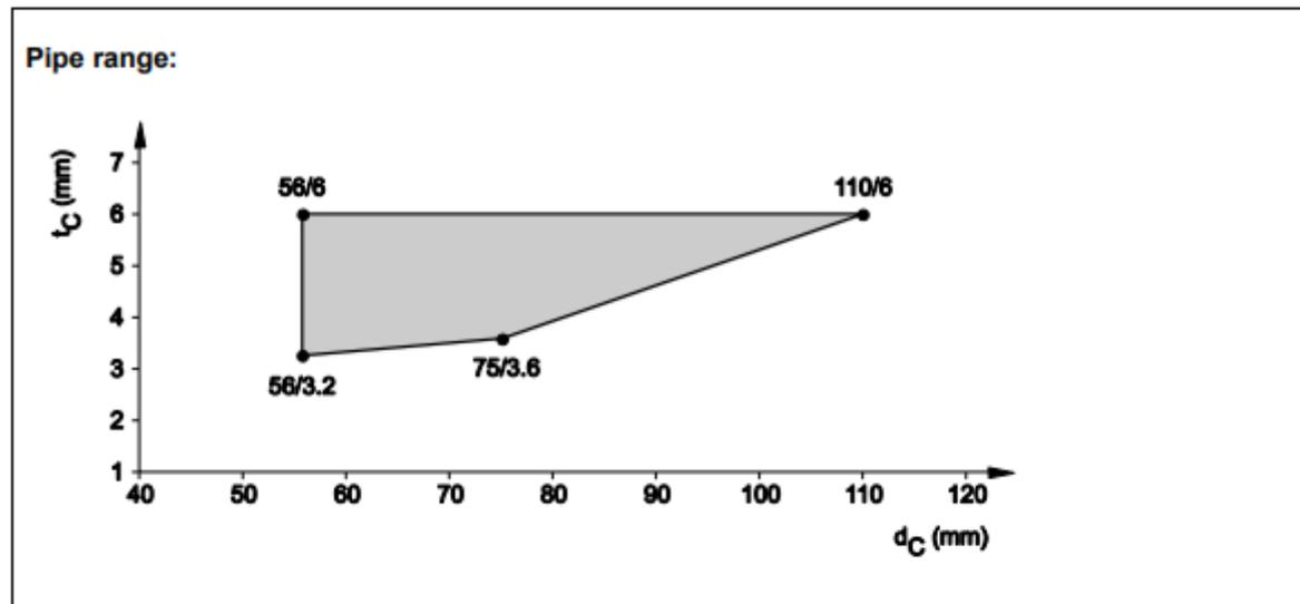
8.6.3.4 Plastic pipes, with 1x 87° elbow in shaft wall system B (refer to 8.6.1.3), EI 90 - U/U
