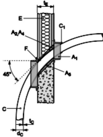
8.3.2.15 PE-X pipe acc. EN 15875 (Rehau Rautitan flex), in flexible wall ( $t_E \geq 100$  mm), pipe group 1, EI 120 - U/C
