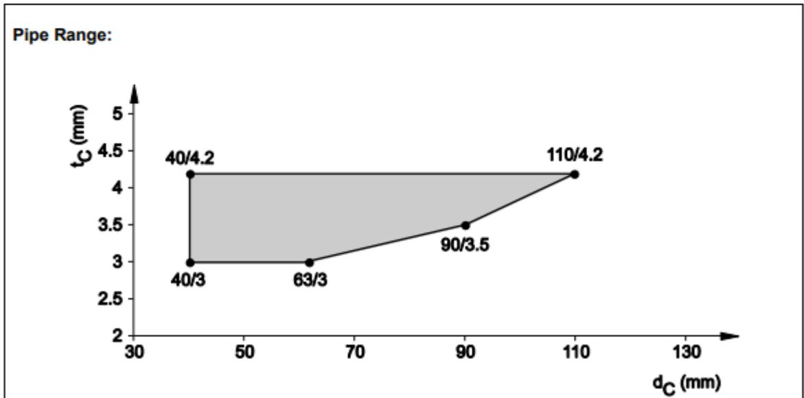
8.3.2.2 ABS-pipes acc. EN 1455, EN 15493 and SAN+PVC-pipes acc. EN 1565-1, in flexible wall, ( $t_E \geq 100$  mm), pipe group 1, EI 90 - U/U
