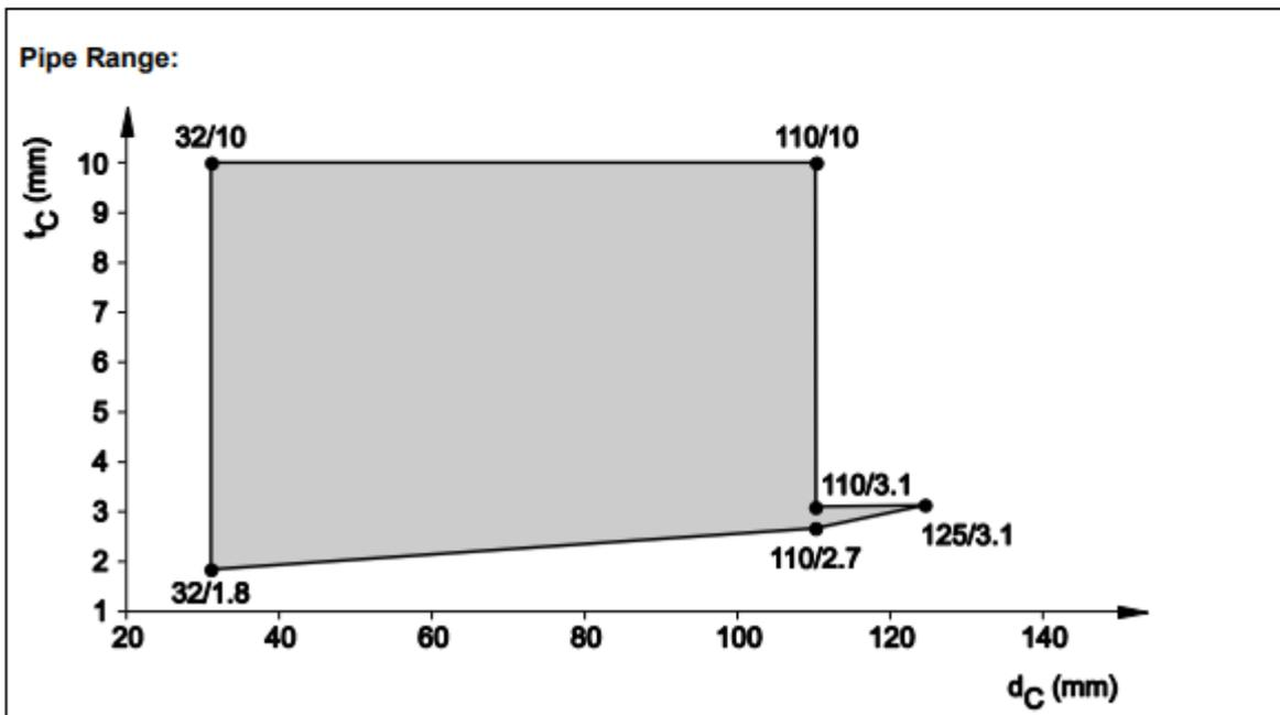
**8.4.2.8 Pipes in rigid wall ( $t_E \geq 100$  mm), pipe group 1, EI 120 - U/U, pipes directly mounted on the wall - zero distance pipe to wall**
