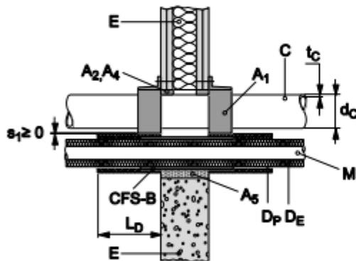
**8.3.2.23.2 Pipes in flexible wall ( $t_E \geq 100$  mm), pipe group 1, EI 90, zero distance between CFS-C EL collar and CFS-B, wrapped around an elastomeric foamed thermal insulation on metal pipe**
