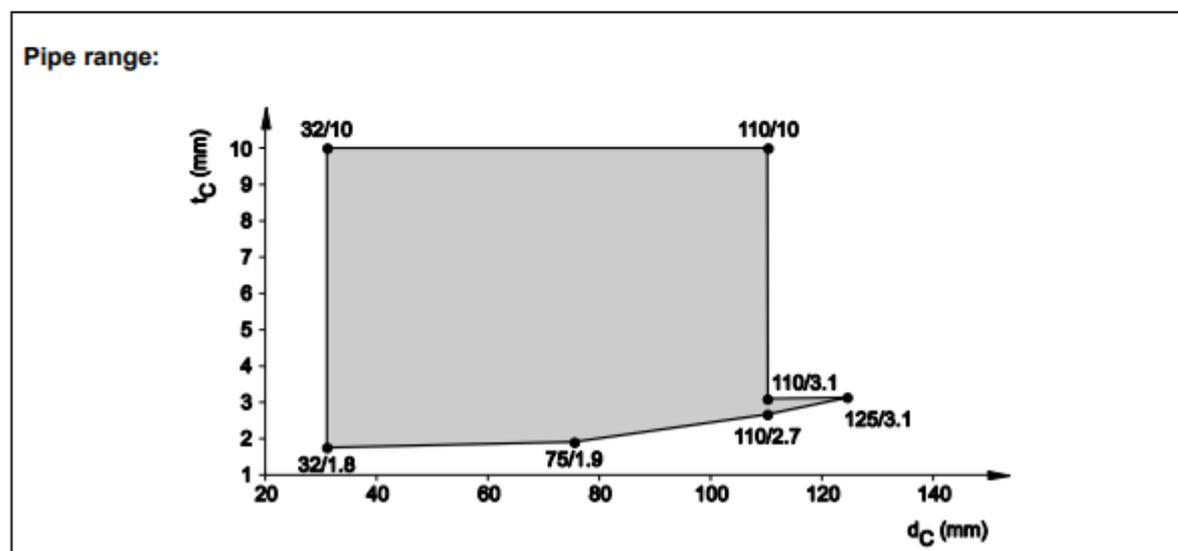
8.5.2.10 PE pipes, non-regulated (Geberit Silent dB20), in rigid floor ( $t_E \geq 150$  mm), pipe group 1, EI 120 - U/U
