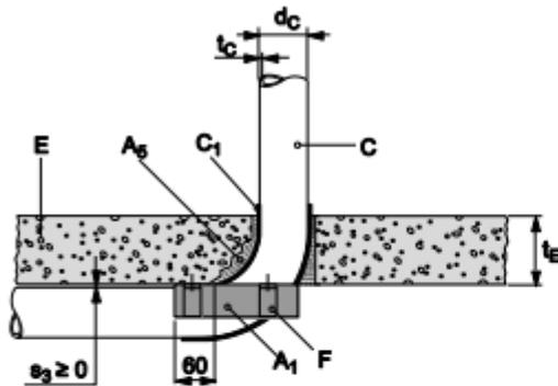
**8.5.2.48 PVC pipes acc. EN 1452-1, EN 1329-1, EN 1453-1, EN 1566-1; DIN 8061/62, EN ISO 15493 in rigid floor ( $t_E \geq 150$  mm), pipe group 1, EI 120 - U/U, Pipe Elbow 87°**
