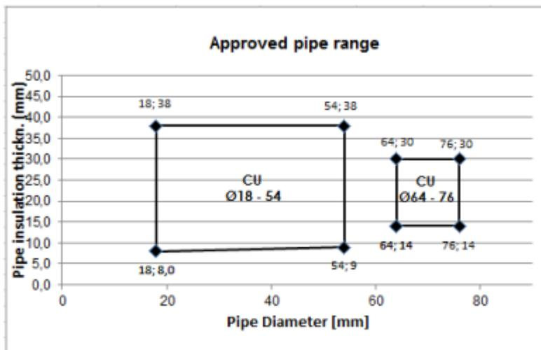
**2.2.11 Copper pipes including metal pipes,
