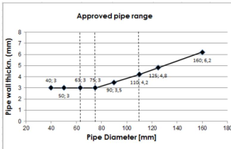
**2.2.1.2 PE pipes according to EN ISO 15494 and DIN 8074/8075****Pipe end configuration: U/C****Distance of penetrations ( $s_1$ ): 0mm / 200 mm (B)**
